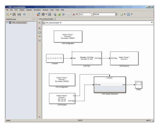
The CAN Configuration block does not connect to any other block. This block configures the CAN channel used by the CAN Receive block to receive the CAN message.
