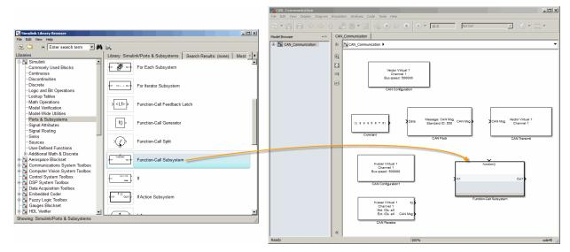
2 Double-click the Function-Call Subsystem block to open the subsystem editor.
