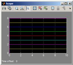
In the graph, the horizontal axis represents the simulation time in seconds and the vertical axis represents the received data value. In the Message Transmit model, you configured blocks to pack and transmit an array of constant values, [1 2 3 4 5 6 7 8], every 0.01 second of simulation time. In the Message Receive model, these values are received and unpacked. The output in the Scope window represents the received data values.
